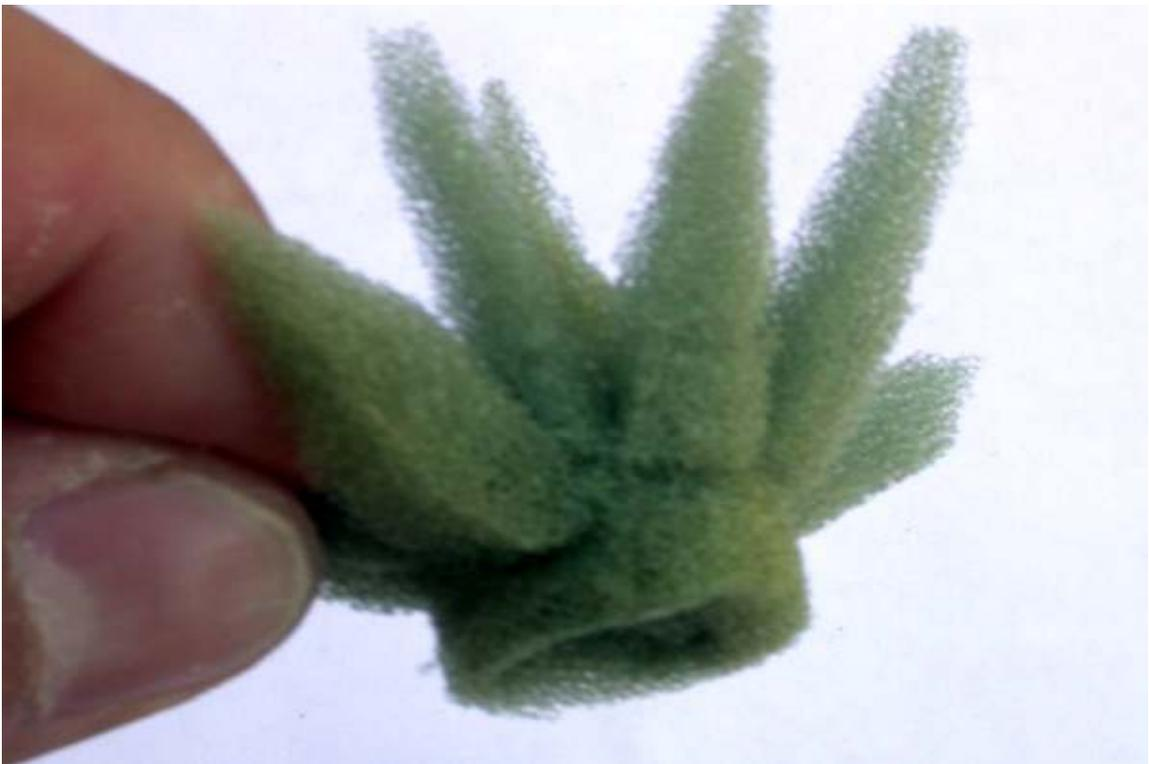
Figure 6. End glued down with CA glue.
