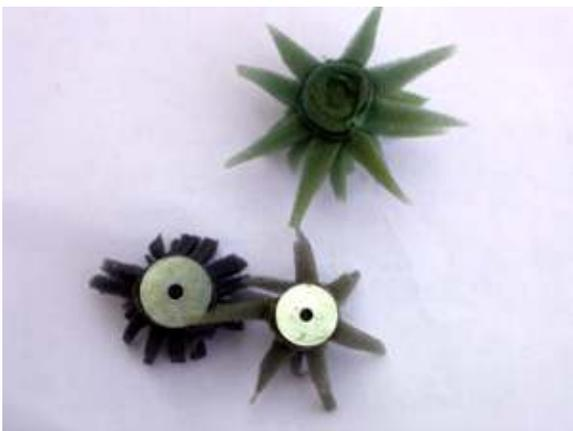
Figure 9. Bottom view of various explosions, some with washers attached.
